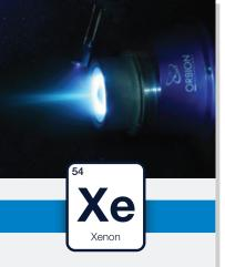
Xenon is a colorless, odorless, nontoxic gas present in the atmosphere. Decades of development experience prove that Xe is the highest-performing EP propellant in the periodic table. Xe is immune from freeze damage, will not contaminate nor damage spacecraft surfaces, has a high storage density (2kg/ liter - 2x greater than liquid water), and is easily metered with proven techniques. Xe is trusted by the most demanding customers.
